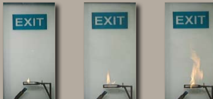
Smoke formation of PLEXIGLAS® (rated B2, normally flammable, to DIN 4102)
