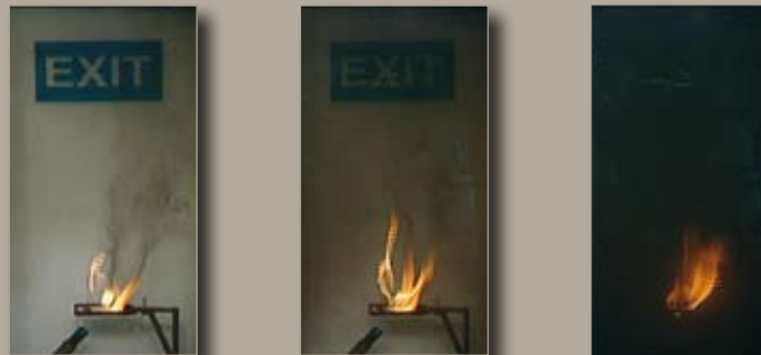
Smoke formation of PVC, PS, SAN, PC, PETG, shown here by the example of PC (rated B1, flame-retardant, to DIN 4102)
